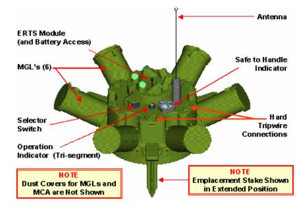
Figure 1: Spider Munition Control Unit (MCU)
